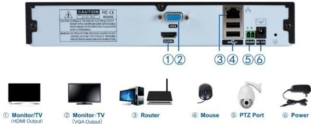
NVR Connections: Diagram 2
