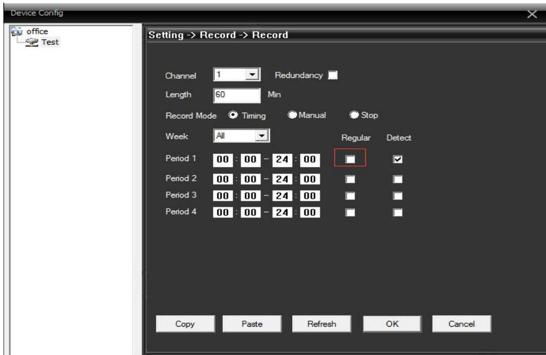
Setup Motion Detection Recording Picture 21
